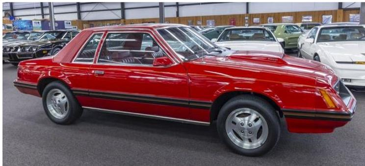
famous. The 2.3 turbo was reported to make 131 hp which was close to 140 hp from the 302, and was available with a four speed in 1979. The Garrett T03 turbo delivered 6 psi of boost. In terms of performance, the 2.3-liter was 70 pounds lighter than the 302 and made almost the same power. The turbo check box also equipped the car with a non-functional hood scoop with "Turbo" badging and a light on the dashboard that glows green under boost and red for overboost.
